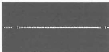
(e) Terminal No. 11. One horizontal line 2.3 v_{p-p} of separated burst ( v_1 = 1.25 v_{p-p} ).
