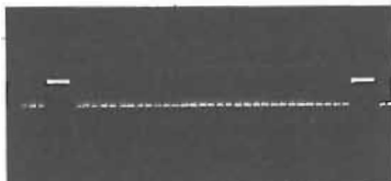
Fig. 19(c) - CA3070 terminal No. 3, 2.0 V_{p-p} oscillator output; one horizontal line, (gated off during burst).
