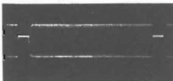
Fig. 19(b) - CA3070 terminal No. 2, 3.5 V_{p-p} oscillator output; one horizontal line, (gated off during burst).
