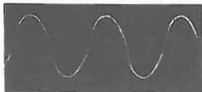
Fig. 20(a) - CA3070 terminal No. 6, oscillator waveform 1.1 V_{p-p} 3.58 MHz.
